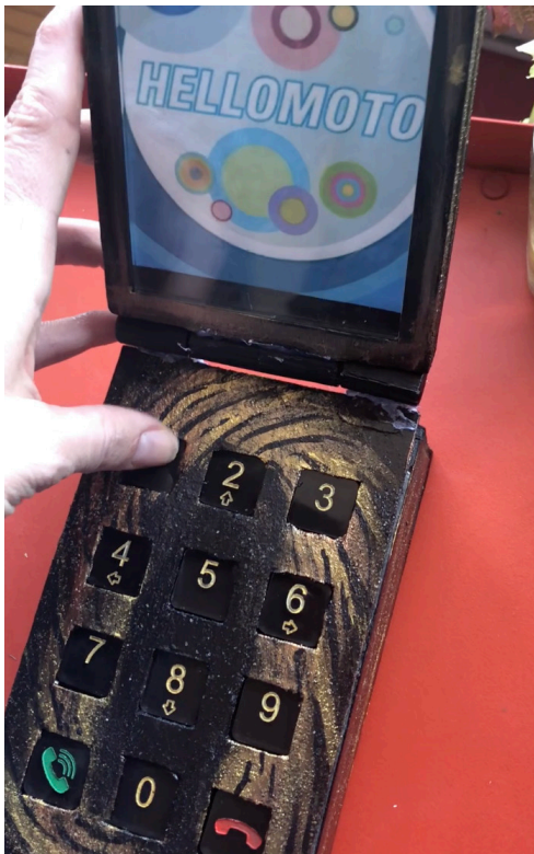
Left image: student designed physical cellphone controller using a Makey Makey kit; right image: screen-based interface of game involving the cellphone controller designed and programmed with javascript..
